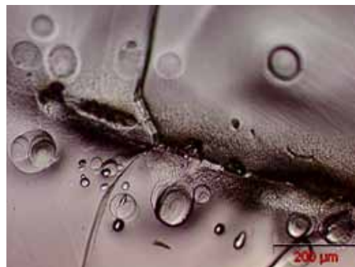
Figure 2a Light microscope image of the hot spot represented in Fig. 1a
