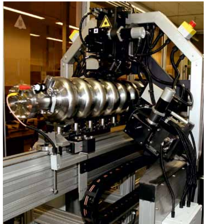
Figure 3 Complete cavity tuning machine with machine housing
