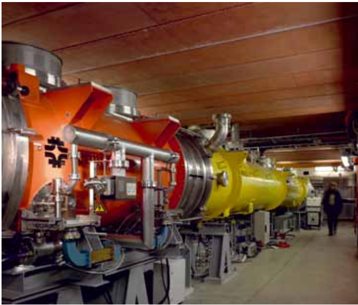
Figure 2 Third-harmonic RF module (red) downstream of first acceleration module (yellow)
