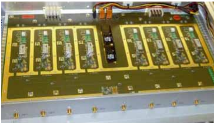
Figure 2 The new RF downconverter for the 3.9 GHz signal of the third harmonic cavities
