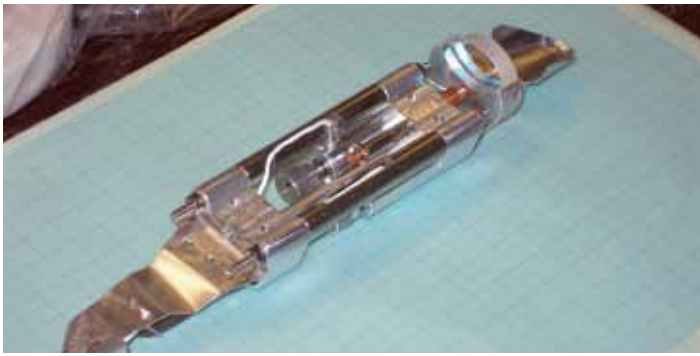
Figure 3 Photo of the end mirror holder with the adopted squiggle motors, suitable for high vacuum and operational under a 5 Tesla magnetic field.
