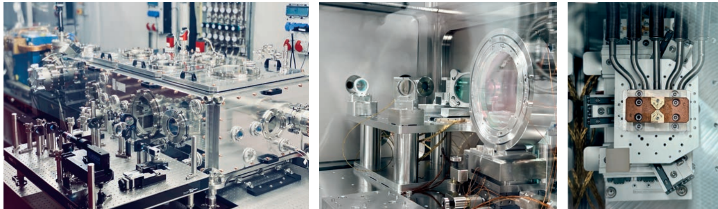
Figure 1 KALDERA’s first laser plasma accelerator MAGMA. Left: Interaction chamber, laser diagnostics and electron beamline. Centre: Final-focusing optics in vacuum. Right: High-average-power plasma source.
