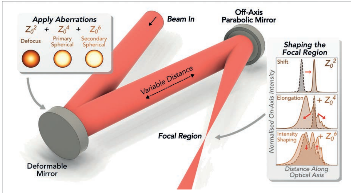
Figure 1 Concept for the scheme: Specific aberrations are added to a deformable mirror placed at a variable distance before the focusing mirror. These aberrations can shape the intensity of the laser pulse in the focal region.
