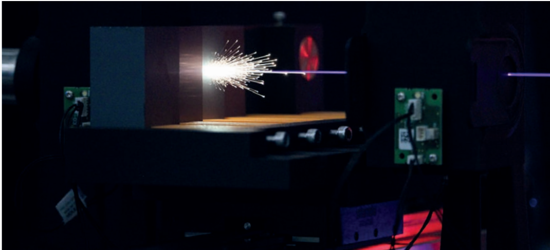
Figure 2 After drilling its way through a 15 mm boron carbide absorber block, a 2.4 keV X-ray beam (coming from the left) creates a “plasma sword” in the ambient air behind the block.
