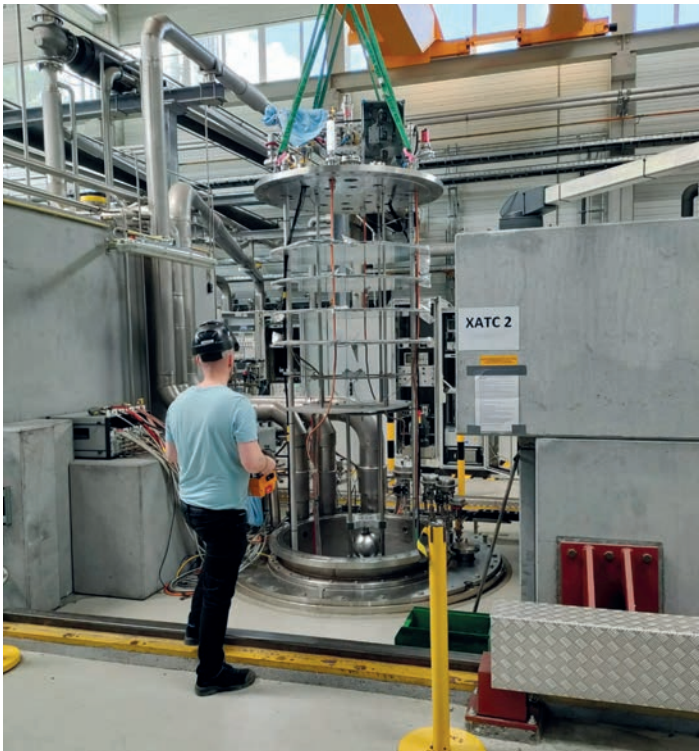
Figure 2 Left: Prototype cavity being installed in a helium bath cryostat in the AMTF facility at DESY. Right (top): Newly developed frame for a set of piezo actuators for generating artificial GW signals and measuring mechanical properties at cryogenic temperatures. Right (bottom): The plot shows the cavity spectrum with a clear peak at the fundamental mode of the cavity, around 2.09974 GHz, and the peak of the signal mode around 11 kHz higher – as intended after tuning. The third peak in between is a driven RF oscillation, generated by inducing an artificial GW with the piezo actuators, which validates the heterodyne detection scheme. The detectable signal is further enhanced if the frequency of the GW (or piezo excitation) matches the frequency difference of the fundamental mode and signal mode f_{\text{drive}} + f_{\text{GW}} = f_{\text{signal}} .
