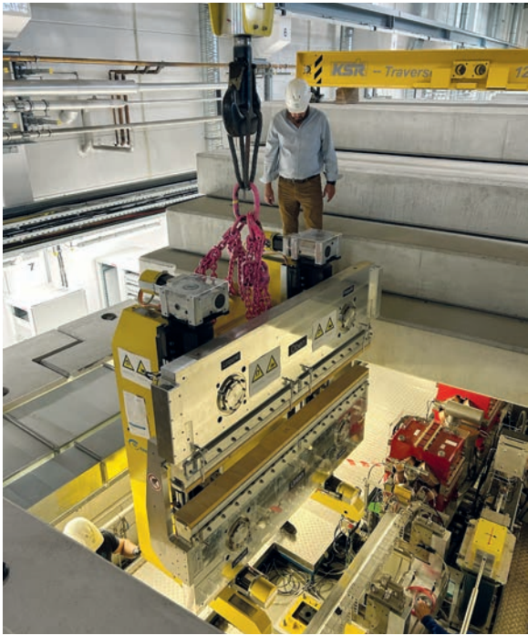
Figure 2 Exchange of the radiation-damaged undulator PU02, located in the PETRA III experimental hall "Max von Laue", in October 2025
