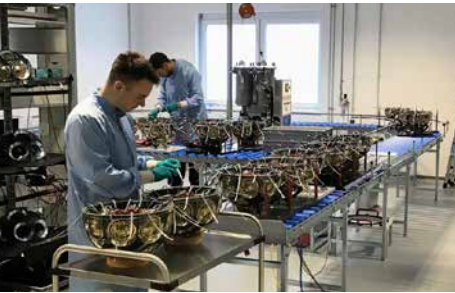
mDOMs for the IceCube Upgrade being assembled under cleanroom conditions at DESY in Zeuthen
