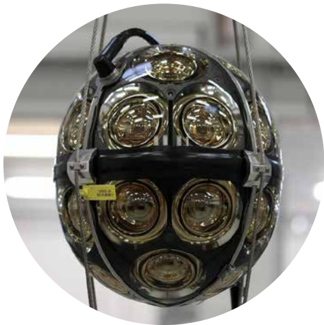
With their 24 light sensors, the mDOMs for IceCube can detect light from all directions.
