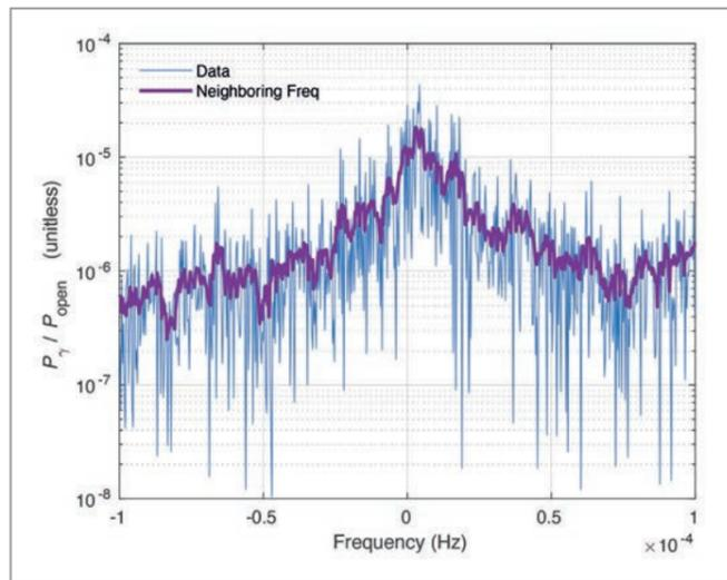
**Figure 1** The plot shows the power of the light detected behind the wall as a function of the frequency difference relative to the correct demodulation frequency for the heterodyne sensing. A signal would show up in the single bin at zero. Data and an interpolation to estimate the background due to stray light are plotted.
