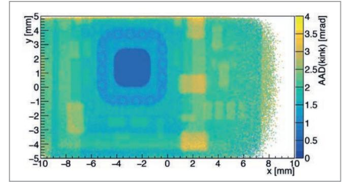
One of these extensions is a module that analyses the material budget of an object. This requires straight tracks to be reconstructed before and after a particle passes the object. The width of the distribution of kink angles between these track pairs is related to the amount and density of material in the investigated object. An example is shown in Fig. 2.
