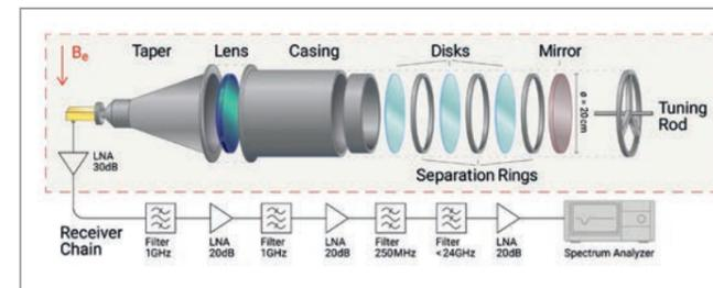
**Figure 3** Exploded schematic view of the MADMAX prototype CB200 (200 mm disk diameter) and the receiver chain used for measurements at CERN. See [2] for details.
