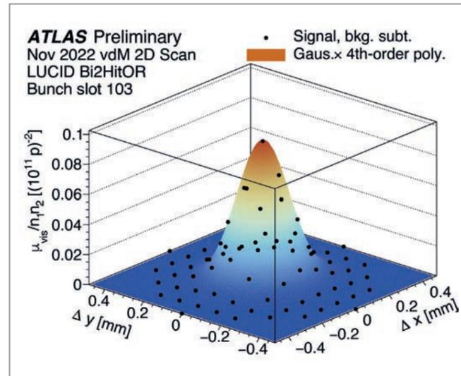
Figure 1 Visible interaction rate per unit bunch population product vs. beam separation in the two-dimensional vdM scan of November 2022, for bunch slot (BCID) 103, using the LUCID Bi2HitOR algorithm
