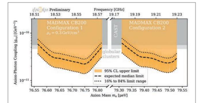
**Figure 4** 95% CL exclusion limits in 0.9 kHz bins (orange) from the 2024 MADMAX axion search with the CB200 prototype using the MORPURGO magnet at CERN, assuming a local axion DM density of  $\rho_a = 0.3 \text{ GeV cm}^{-3}$ . Limits are compared to the helioscope experiment CAST (dark grey) as well as to globular cluster limits (light grey). See [2] for details.
