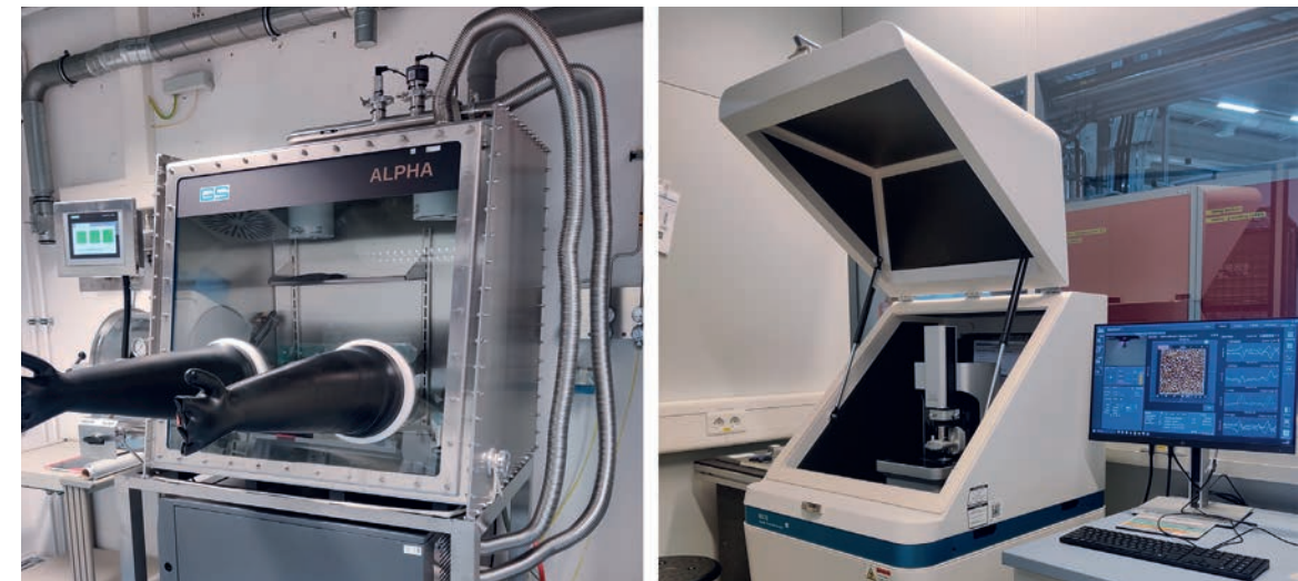
Figure 7 The new glove box in the chemistry laboratory in the PETRA III experimental hall 'Ada Yonath' (left) and the new atomic force microscopy instrument (Park SmartScan) in the experimental hall 'Max von Laue' (right). (Credit: DESY)
