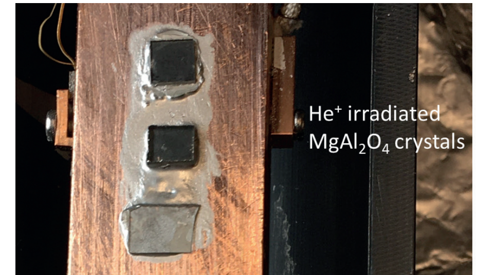
Figure 2 The photo shows three different samples on the sample holder (Credit: DESY).
