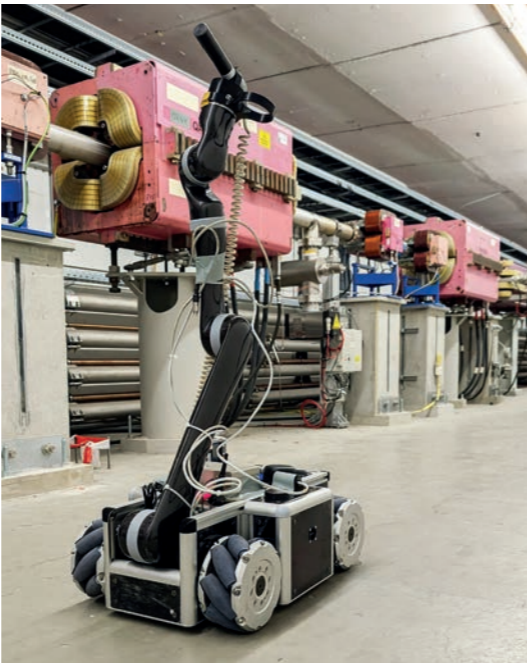
Figure 1 Left: The MIRA3 robot in front of the PETRA III East hall after unboxing. Right: MIRA3 with a mounted radiation detector in the PETRA III tunnel.
