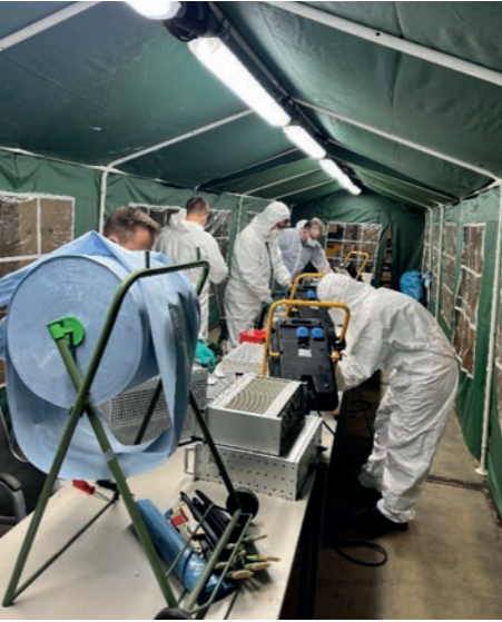
A complete cleaning line for removing soot and extinguishing-powder residues from electronic components was set up in the Test Beam hall. Thanks to the concerted effort, damage was minimised, everything cleaned up, and user operation resumed.
