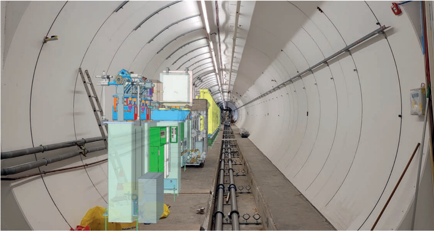
Figure 1 Illustration of the new externally seeded FLASH1 beamline fitted into the emptied and renovated tunnel. Most prominent are the yellow support structures that hold the new force-compensated APPLE-III undulators, which make it possible to generate arbitrarily polarised beams at variable wavelengths.
