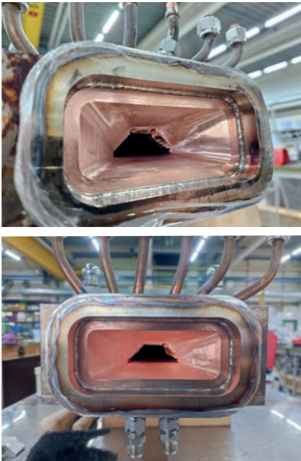
Figure 2 View inside the damaged absorbers of the wiggler sections West (top) and North (bottom)
