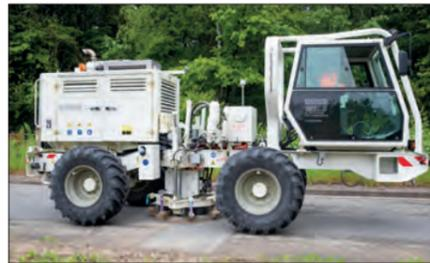
Using a fibre-optic network, the WAVE collaboration measured vibrations caused by a vibrotruck on the DESY campus.
