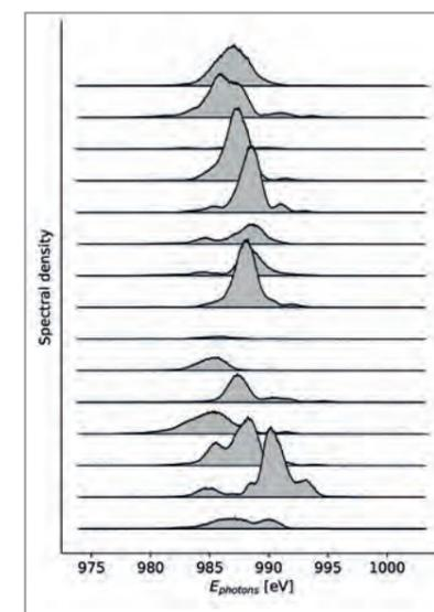
**Figure 3** Left: Ten consecutive measurements of nearly single-spike X-ray spectra at an averaged pulse energy of about 600  $\mu$ J. Right: Simulations reproducing the experimental results.
