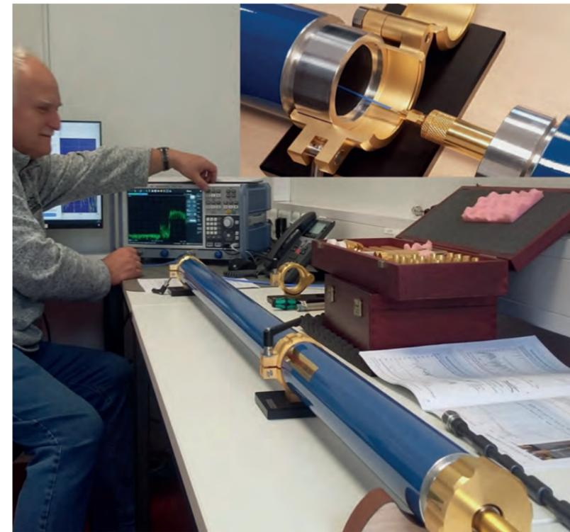
**Figure 2** Setup for measuring the screening attenuation of an RF cable
