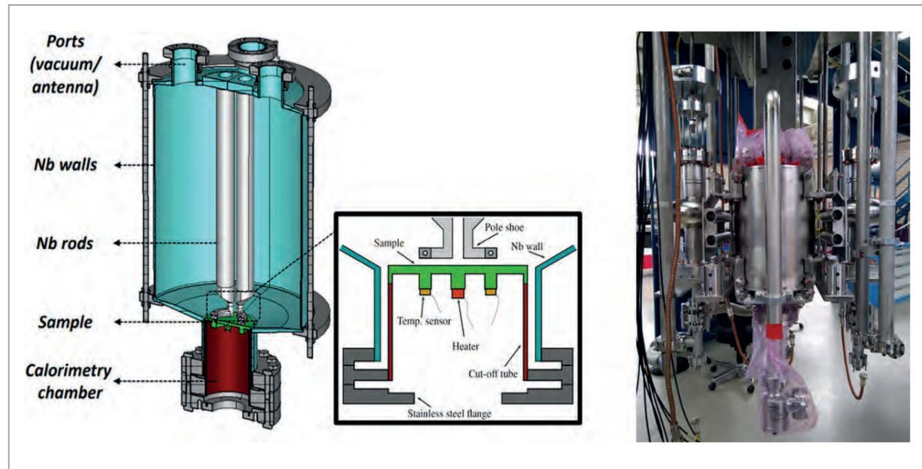
**Figure 1** Left: Schematic view of the QPR. The inset shows a cross section through the sample and the bottom part of the rods [1]. Right: QPR installed and vacuum connections assembled for the first cooldown to 1.5 K at the Accelerator Module Test Facility (AMTF) at DESY.
