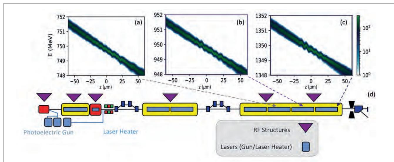
**Figure 1** Start-to-end simulations Part I: In the accelerating structures and bunch compressor sections of the beamline, the simulations are performed with *Impact-Z* and *elegant* or *SelaV*. The beams with 400 pC charge used for the three energy working points of (a) 750 MeV, (b) 950 MeV and (c) 1350 MeV are shown along the accelerator layout (d).
