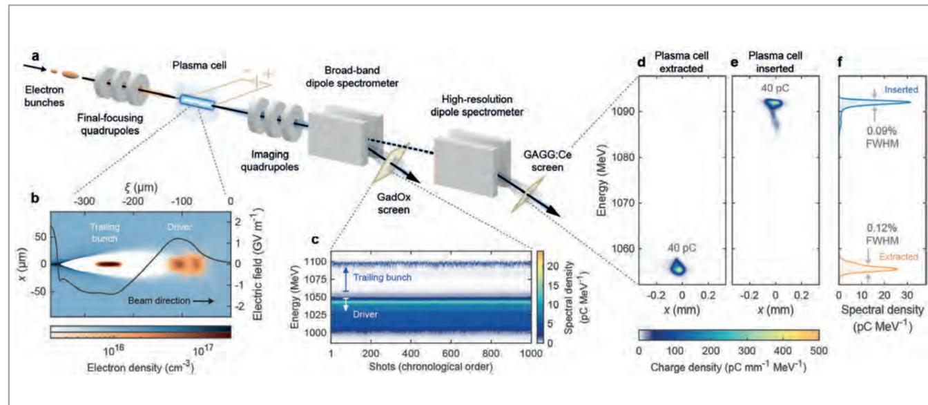
Figure 1 a) Experimental setup at FLASHForward. b) Insets showing the simulated, beam-driven plasma wake. c) Measured, highly stable energy spectrum of the accelerated beam. d) Spectrometer images demonstrating both charge and energy spread preservation. From [3].
