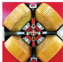
Quadrupole magnet from DESY's synchrotron radiation source PETRA III. Such magnets are used to control the size of the electron beam that zips around the 2.3 km circumference storage ring. In the PETRA IV upgrade, these magnets will be smaller and there will be many more of them to keep the beam size as small as possible throughout the facility. This will result in 500 times brighter X-rays. Stay tuned for the future!
