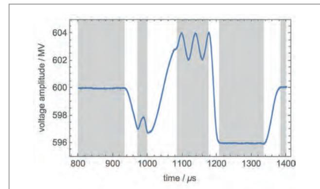
Figure 2 Demonstrated voltage amplitude (RF pulse flat-top, Station A2) with five Beam Regions (grey zones). BR 2 and BR 3 have arbitrary modulation. The white zones are the so-called transitions.
