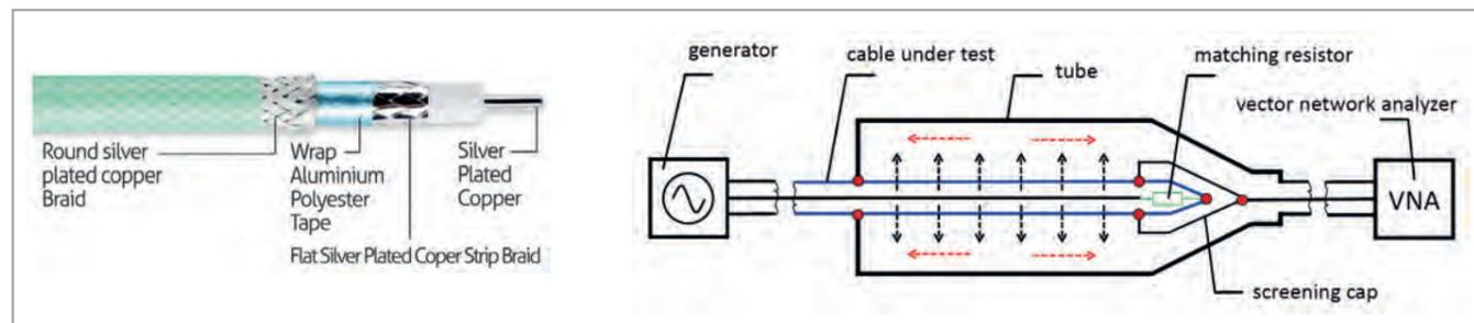
**Figure 1** Left: Layer structure of a high-frequency cable with two layers of shields. Right: Simplified block diagram of the setup for measuring the radiation passing the shield of a high-frequency cable.
