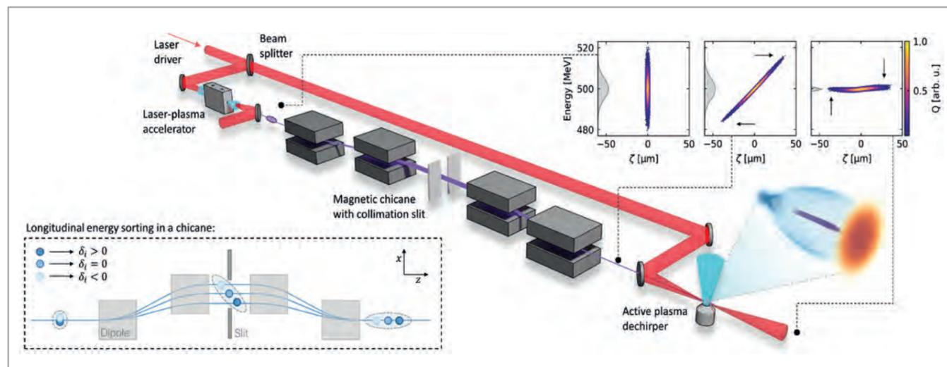
Figure 1 General overview of the energy compression concept showing the main components and beam manipulations. Adapted from [4].
