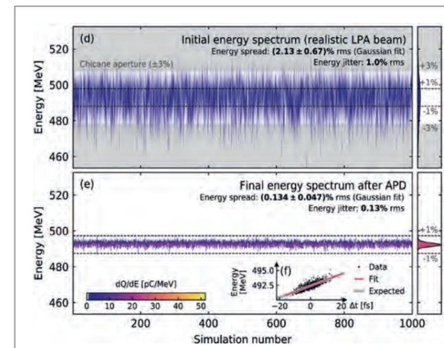
Figure 2 Shot-to-shot energy spectrum of the LPA beam before (top) and after (bottom) the energy compression beamline. Adapted from [4].
