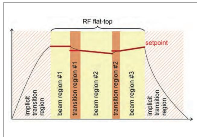
Figure 1 Sketch of the typical RF pulse form, showing the Beam Regions concept
