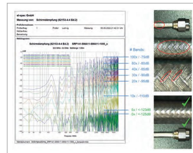
**Figure 3** Screening attenuation of a conformable RF cable for different numbers of mechanical bends. The attenuation degrades after some bends due to microscopic cracks of the soldered shield braid.
