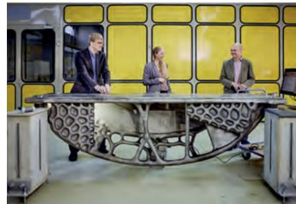
The team of physicists, biologists and engineers developed various novel girder prototypes inspired by nature, based on the structural principles of tiny aquatic plankton organisms, for low-vibration, lightweight constructions as support frames for the PETRA IV magnet optics. However, the shape of the prototype ultimately depends on the magnet optics that are being developed in parallel, and manufacturing costs also play a role.
