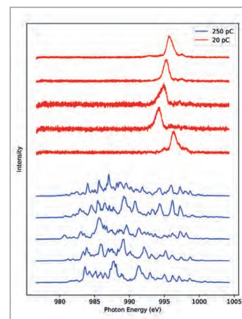
**Figure 2** Selected X-ray spectra for nominal (250 pC) and low-charge (20 pC) electron bunches with optimised compression
