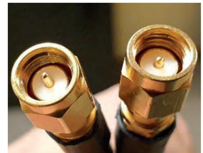
**Figure 4** Movement of inner connector pins due to stress
