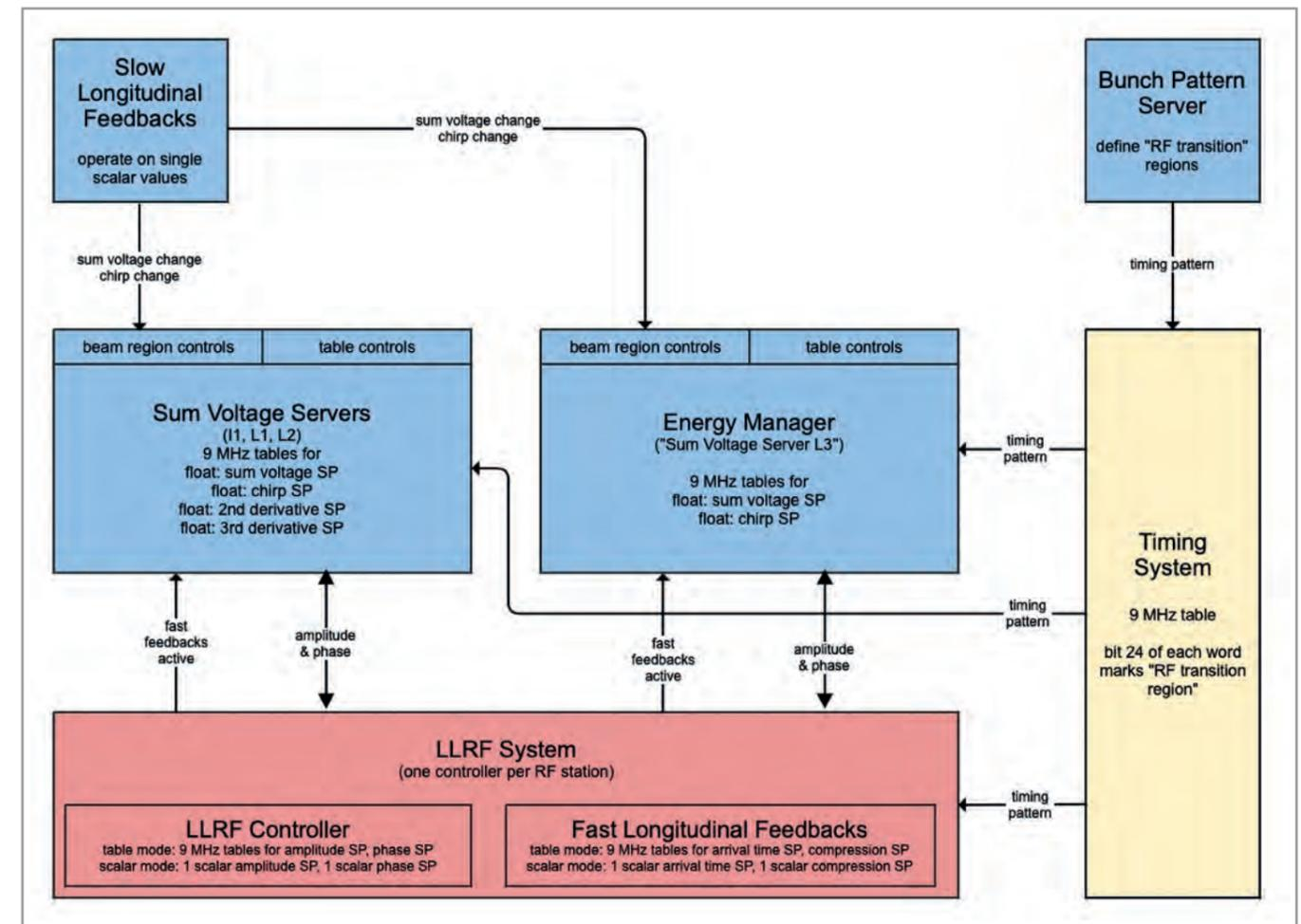
Figure 3 Control system architecture to support Beam Regions
