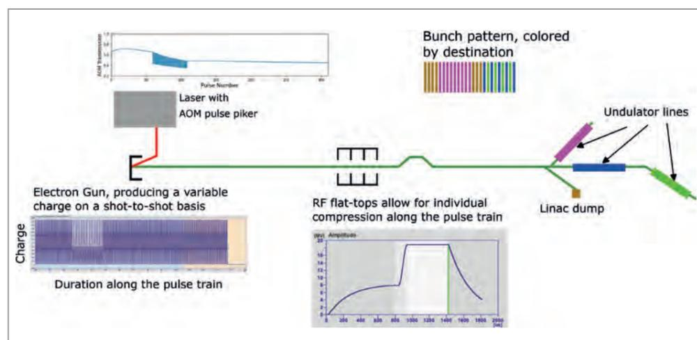
**Figure 1** Schematic layout of the European XFEL with its electron bunch trains feeding the three undulator lines. The laser AOM absorber located close to the electron gun makes it possible to arbitrarily shape the charge profile of the electron bunches. The modulated RF flat-top enables individual bunch compression along the train. Note the different time scales of the two options, which make them appropriate for different delivery modes (depending on the destination of the bunches).
