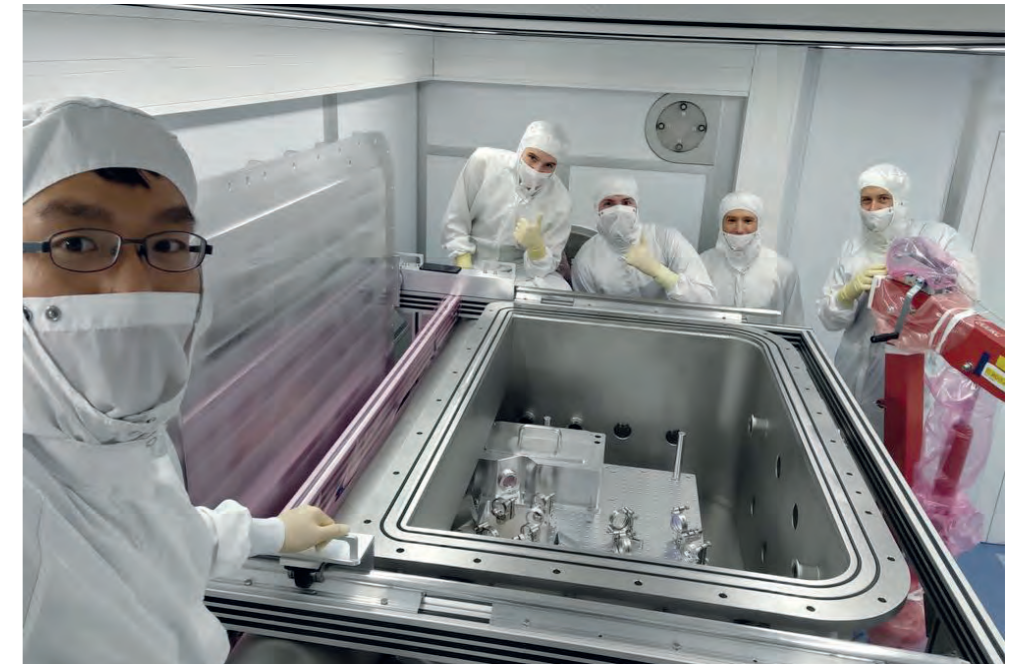
Figure 2 ALPS II optics team members with the vacuum chamber housing the central optical bench
