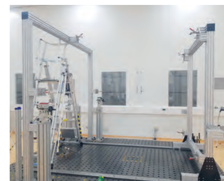
Figure 4 Final DD assembly tooling. The left part for disk assembly comprises a fixed Dee portal and precision stages to align the second Dee. The rail frame on the right serves as pick-up for the disk and the final disk-to-disk alignment.
