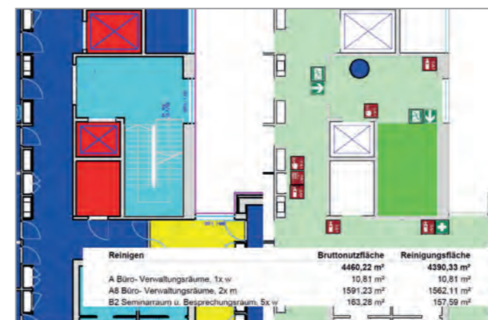
Figure 3 Floor plan with color codes for room type and summary of areas for cleaning contracts, and the same plan rendered for escape and rescue planning
