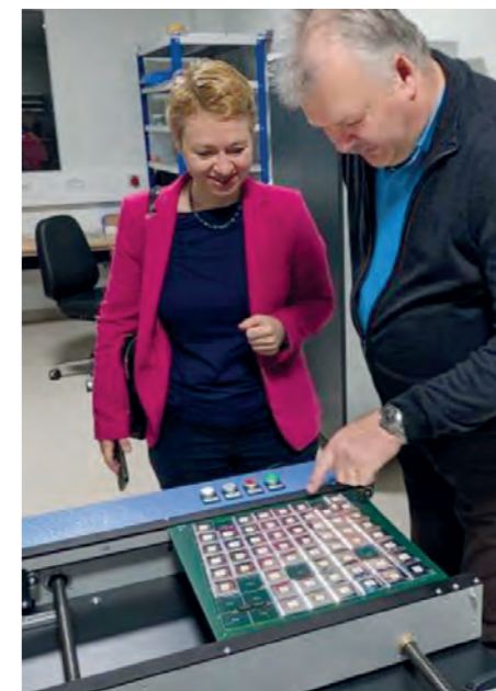
Figure 3 Beate Heinemann, Director of the DESY Particle Physics division, and Reinhard Schapheit from the DESY ZE group inspect a tileboard after gluing of the tiles with the pick-and-place machine.
