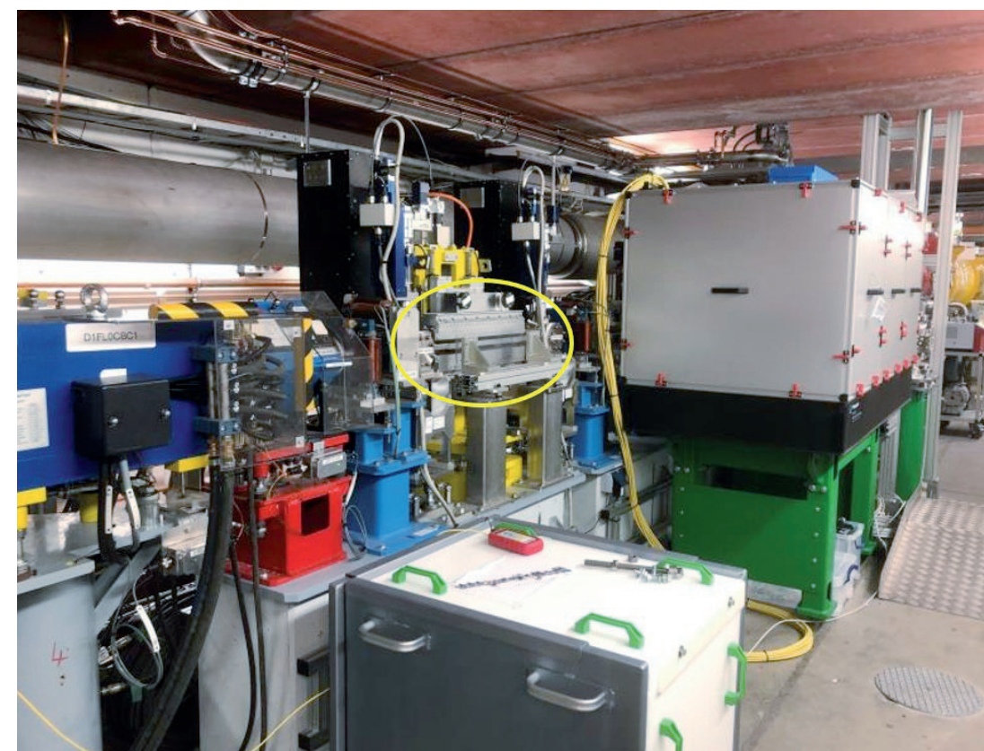
Figure 2 Laser heater undulator (yellow circle) and a large box with a laser table for optical components (right of it on green supports) to couple the laser pulses into the electron beamline. In the background at right, the yellow first accelerating module in the FLASH tunnel is visible.
