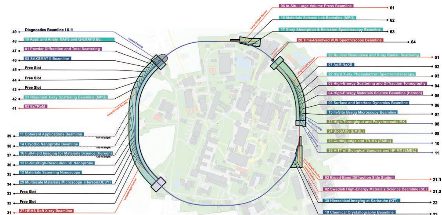
Figure 2 Distribution of the currently planned PETRA IV beamlines in the new experimental hall (in blue-green, left) and in the already existing three experimental halls (in light green, right) in the eastern part of the storage ring (blue line). The beamlines in the eastern halls will be the first to be put back into operation after the PETRA IV accelerator complex is commissioned in 2029.
