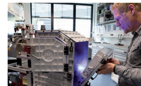
Mobile X-ray tomographic scanner, developed at DESY, is designed to decipher closed cuneiform tablets.
