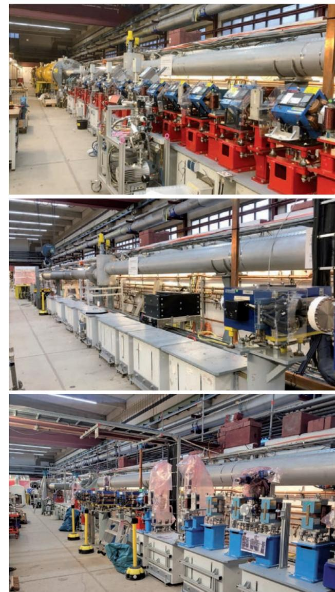
being warmed up from their 2 K operation temperature, allowing for the exchange of two out of seven modules. They were replaced by two new, state-of-the-art modules following the European XFEL design (Fig. 2). The exchange will increase the maximum electron energy of FLASH by 100 MeV to a total of 1.35 GeV. This will result in shorter photon wavelengths becoming available to users and extend the feasible experimental applications.
