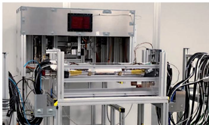
Figure 3 First fully instrumented half-shell of the newly constructed PXD2 (top). After mounting the detector on a dummy beam pipe, it will be subjected to a thorough test procedure using a special source setup installed in the cleanroom of the Helmholtz detector laboratory in the HERA West hall at DESY (bottom).
