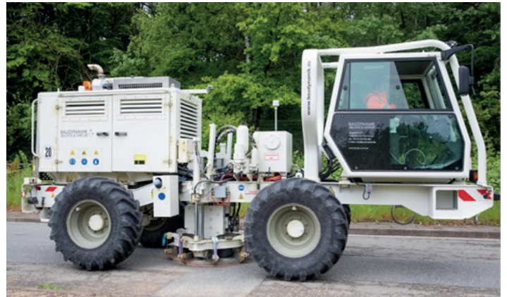
The WAVE collaboration used telecommunications fibres to localise vibrations generated on the DESY campus by a Vibrotruck.
