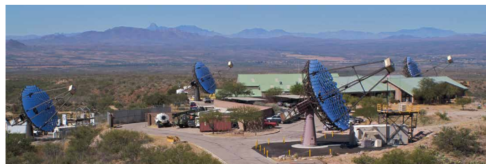
The VERITAS array of imaging atmospheric Cherenkov telescopes for the observation of cosmic gamma rays
