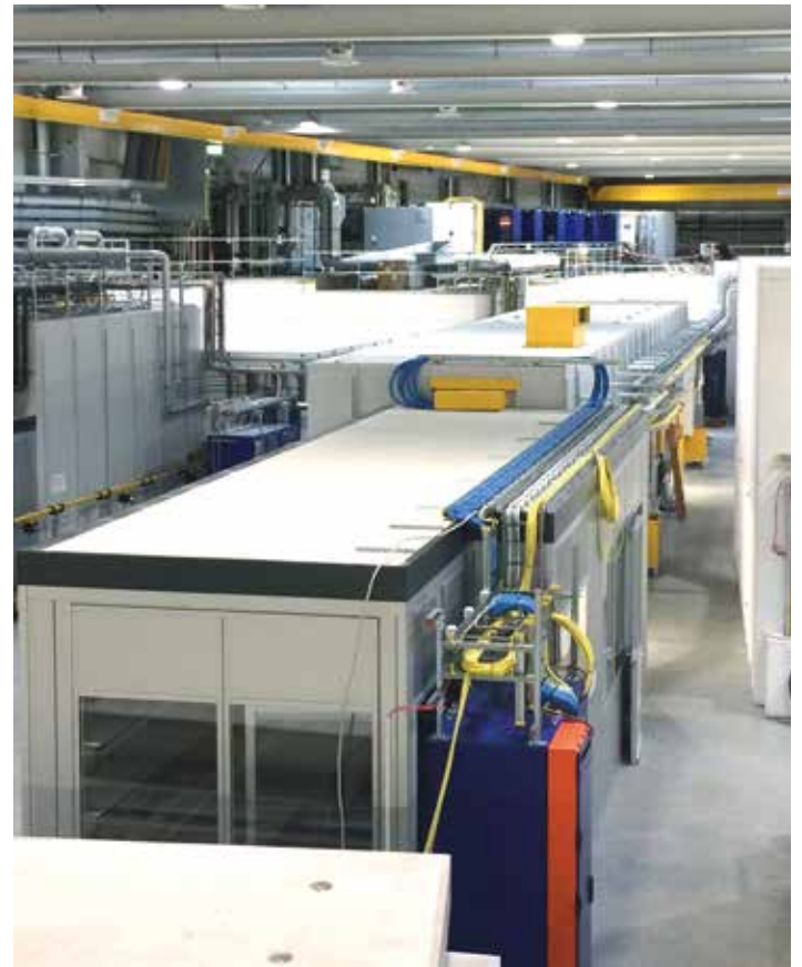
Figure 7 Left: image of the open P62 optics hutch with girders installed. Right: view on the PETRA III beamline P62. In the front the control hutch, in the back the experimental hutch.
