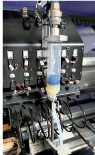
Figure 3 New dispensing tool within the SMD placement automat, with the glue cartridge in the foreground
