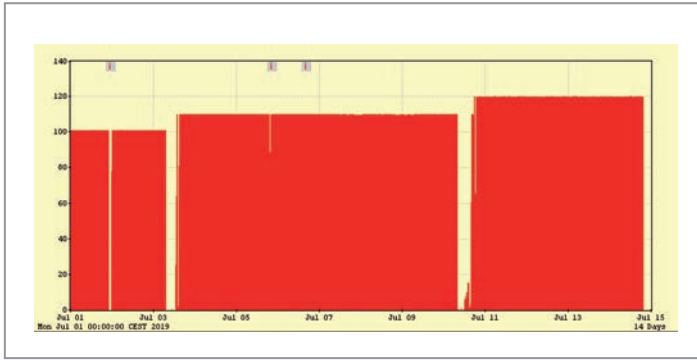
Figure 3 History of the PETRA III beam current from 1 to 15 July 2019. The beam current in the 480 bunch mode was increased to 120 mA.
