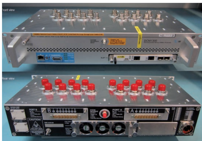
Figure 3 2U 19-inch packaged drift compensation module for 16-cavity probe signals. Front and rear view.
