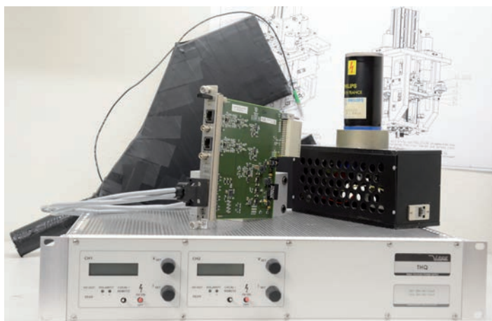
Figure 4 Readout electronics for the photomultiplier signal: Wire scanner detector RTM (left) and photomultiplier tube with base (right) standing on a commercial off-the-shelf high-voltage power supply. The photomultiplier signals are relayed to the RTM using differential cables with standard RJ45 connectors. A black wrapped-up scintillating paddle is partially visible in the background.
