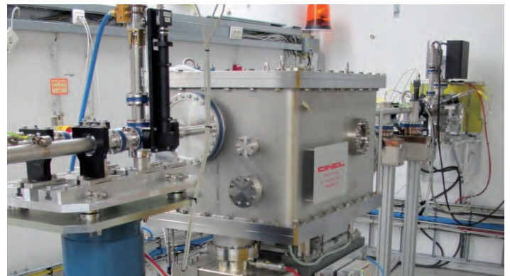
Figure 5 (Top) Single-bounce Laue monochromator at the PETRA III beamline P21 (side station). (Bottom) Diffraction pattern of Si powder taken at 100 keV using a 2D Si-detector (sample to detector distance 1 m).
