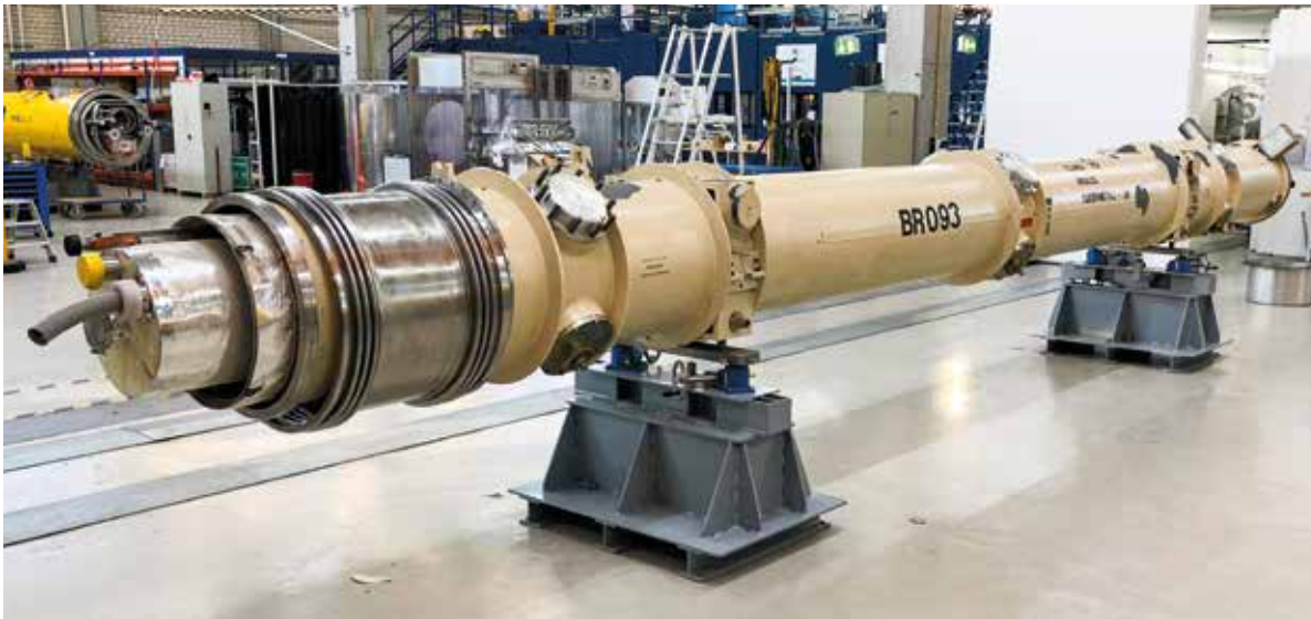
Figure 2 Straightened HERA dipole for the ALPS II experiment during measurements and testing at DESY
