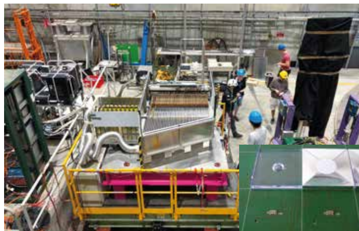
Figure 1 AHCAL prototype installed in the SPS test beam area at CERN. Insert: Detailed view of the SiPM-on-tile design.
