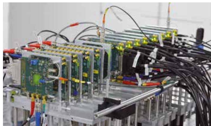
Figure 1 Eight Mu3e sensor layers together with two scintillating tiles in a custom tracking telescope
