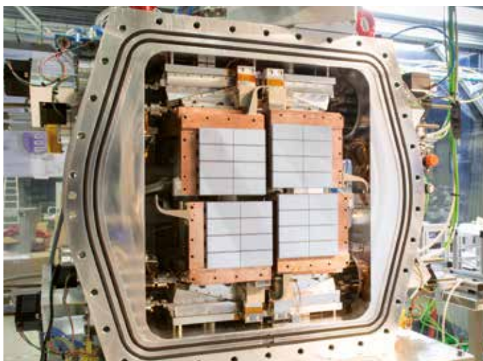
Figure 1 Entrance window side of the DSSC X-ray imager based on mini-SDDs
