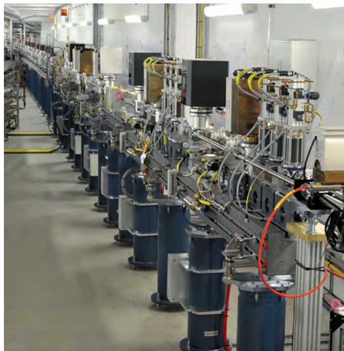
Figure 1 New 2 m undulators for beamlines P22, P23 and P24 in the PETRA III ring tunnel (left). Completed frontend of the PETRA III beamline P21 with a length of 90 m from the undulator source to the tunnel wall (right).
