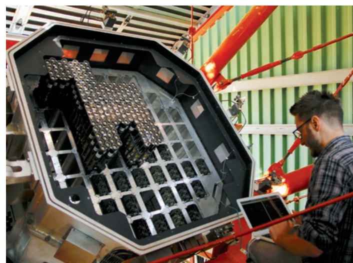
Figure 2 Commissioning the new front-end electronics of one of the H.E.S.S. I cameras
