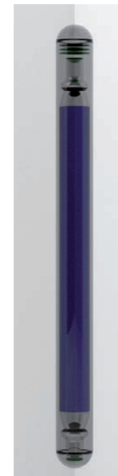
Figure 3 Wavelength-shifting optical module (WOM) for the IceCube-Gen2 project. The light collected in a wavelength-shifting coated tube (blue) is transported to two small PMTs at the ends of the tube. The whole setup is protected by a UV-transparent quartz pressure housing.
