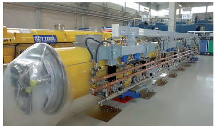
Figure 4 Module waveguide distribution connected to one accelerator module
