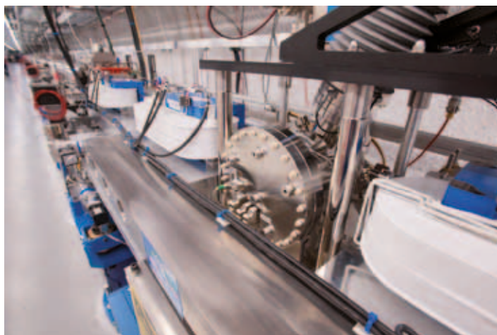
The chamber containing the diamond crystal used for self-seeding at SLAC
