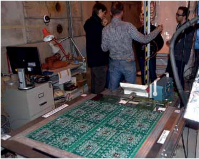
Figure 2 Installation of an HCAL readout layer with 576 scintillator tiles and SiPMs into the CALICE tungsten stack in the SPS beam at CERN
