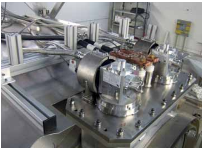
Figure 1 Close-up view of the two cryo-coolers installed on the PCMAG magnet. The coolers are pneumatically operated and operate as a closed system.
