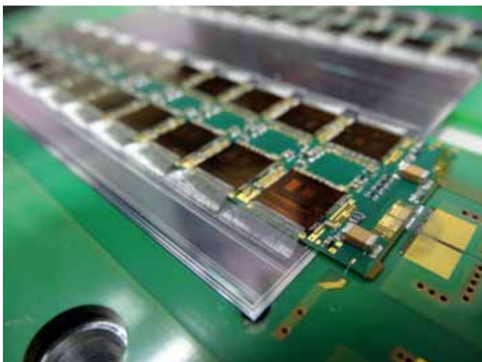
Figure 4 ATLAS single-sided silicon strip module for the HL-LHC detector upgrade
