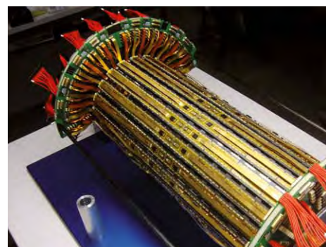
Figure 1 The present three-layer BPIX consists of 672 modules with 66 560 pixels each and 96 half-modules. (Courtesy: PSI)
