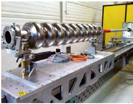
Figure 2 The automated cavity inspection tool OBACHT. A cavity is placed on a sledge driven by a linear motor; the camera is housed at the end of the rod in the background and can be rotated by 360° using the torque motor drive. (Courtesy: Heiner Müller-Elsner)
