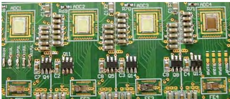
Figure 2 Four fast 10-bit ADC ASICs with eight channels from UST Cracow mounted on the readout board
