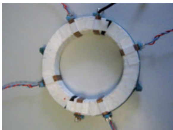
Figure 1 Ferrite core with two test windings and four output windings
