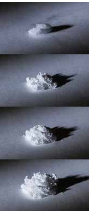
When HDA ice is converted into LDA ice, the volume of ice spontaneously increases by about a quarter.
