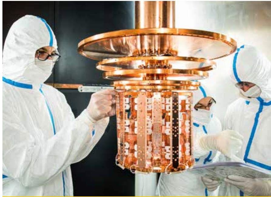
The Cryogenic Rare Event Search with Superconducting Thermometers (CRESST) experiment is located 1400 metres beneath Italy's Gran Sasso mountain massif, where it searches for tiny temperature fluctuations that can be triggered by the rare collision of a dark matter particle. Work on the central detector part must be conducted under cleanroom conditions.
