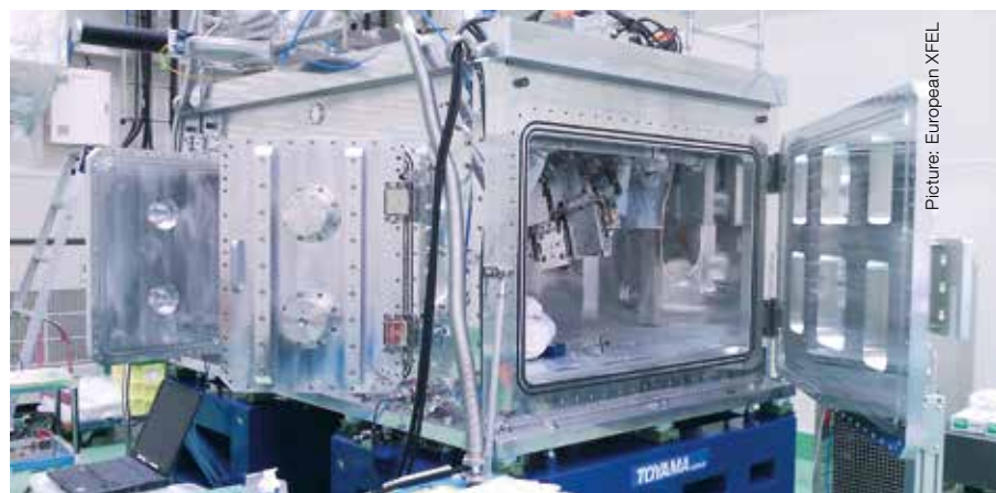
Experimental chamber of the High Energy Density Science instrument at the European XFEL X-ray laser.
