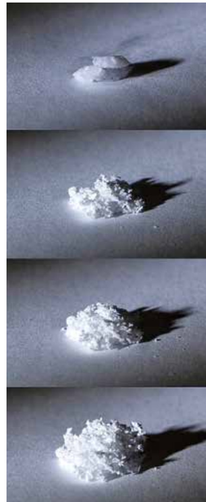
When HDA ice changes to LDA ice upon warming, it suddenly grows in volume by about a quarter, as had been observed before.
