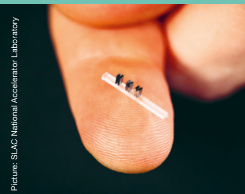
Three “accelerators on a chip” made of silicon are mounted on a clear base.
