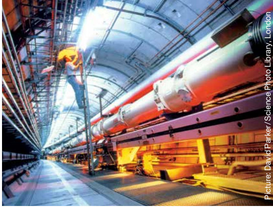
The HERA particle accelerator consists of a proton ring (above) and an electron ring (below).
