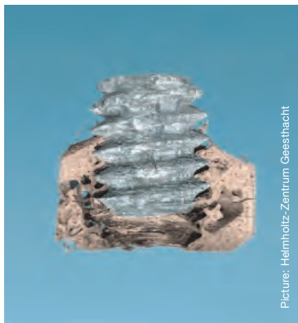
Real-time tomography serves to investigate dynamic processes such as the degradation of a bone screw made of a new type of magnesium alloy.
